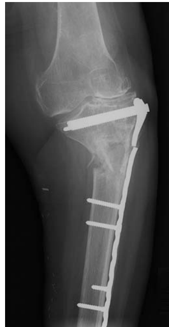
Fig. 3 Bridge plating with plate fatigue failure through unplugged locking screw hole.
